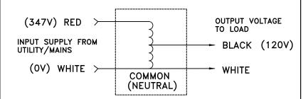
Note: "F" version has an internal auto reset 110°C thermal protector in series with the "RED" input lead.
