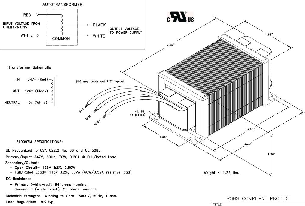
Efficiency: 86% typ. @ 347Vin, 60VA load.
